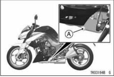
A. Engine Oil Drain Bolt
