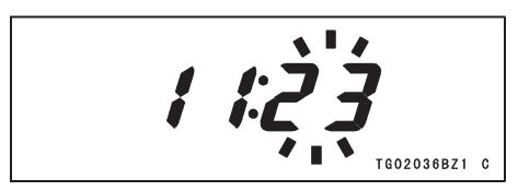
Push the lower button. Both the hour and minute displays start blinking again.  Push the upper button. The displays stop blinking and the clock starts working.
