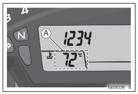
A. Lap Counter/Coolant / Intake Air Temperature Meter
