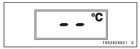
When the coolant temperature rises to above 40°C (104°F), the numerical value of the coolant temperature at the present state is displayed.
