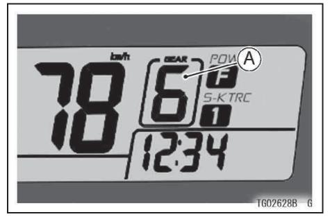
A. Gear Position Indicator (Normal mode)
