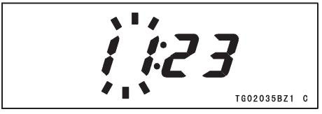
Push the lower button. The hour display stops blinking and the minute display starts blinking. Push the upper button to advance the minutes.
