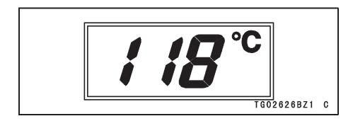
If the coolant temperature rises to above 120°C (248°F), "HI" is displayed and starts blinking and the red warning indicator light also goes on. This warns the operator that the coolant temperature is too high. Stop the engine and check the coolant level in the reserve tank after the engine cools down.
