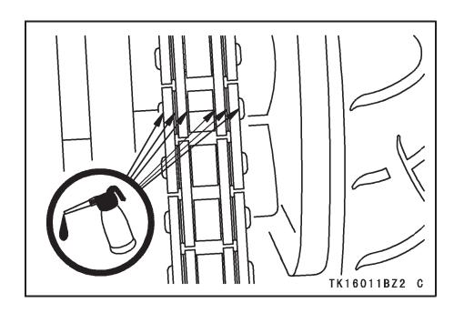
• If the chain is especially dirty, clean it using diesel oil or kerosine and then apply oil as described above.
