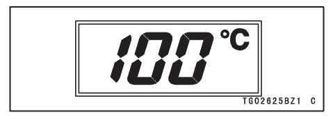
• If the coolant temperature rises to above 115°C (239°F) and below 120°C (248°F), the numerical value of the current coolant temperature starts blinking and the red warning indicator light also goes on. This warns the operator that the coolant temperature is high.
