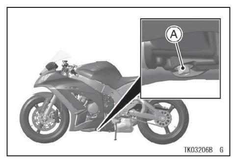
A. Engine Oil Drain Bolt
