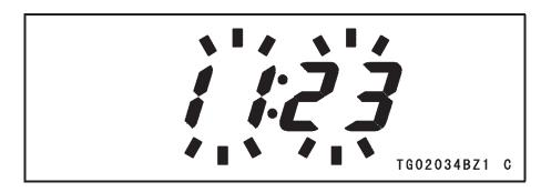
Push the lower button. The hour display only blinks. Push the upper button to advance the hours.
