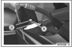
A. Spring Preload Adjuster B. Adjuster Position
