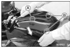
A. Projection B. Hook Fasteners
