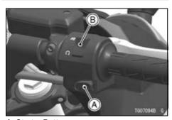
A. Starter Button **B. Engine Stop Switch**
