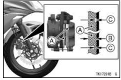
A. Front Brake Pads **B. Lining Thickness**
