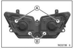
A. Horizontal Adjusters B. Vertical Adjusters
