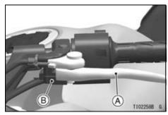
A. Clutch Lever B. Starter Lockout Switch
