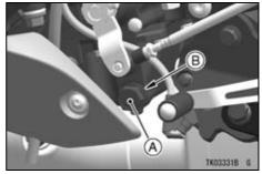
A. Engine Oil Drain Bolt B. Gasket
