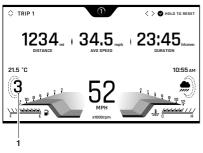
1. Gear position display (third gear displayed)
