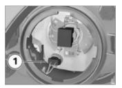
• Remove bulb holder **1** from the headlight housing.
