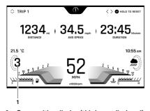
1. Gear position display (third gear displayed)
